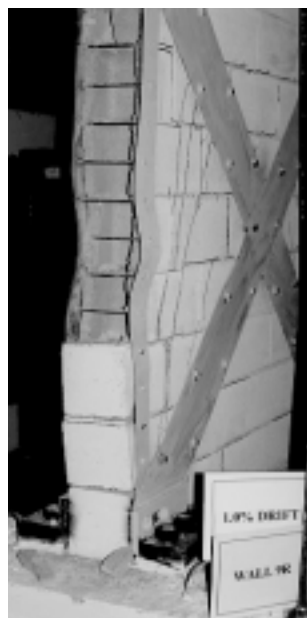
Fig. 10. Wall 9R: at the end of 1.0% drift, global buckling of vertical steel strips
