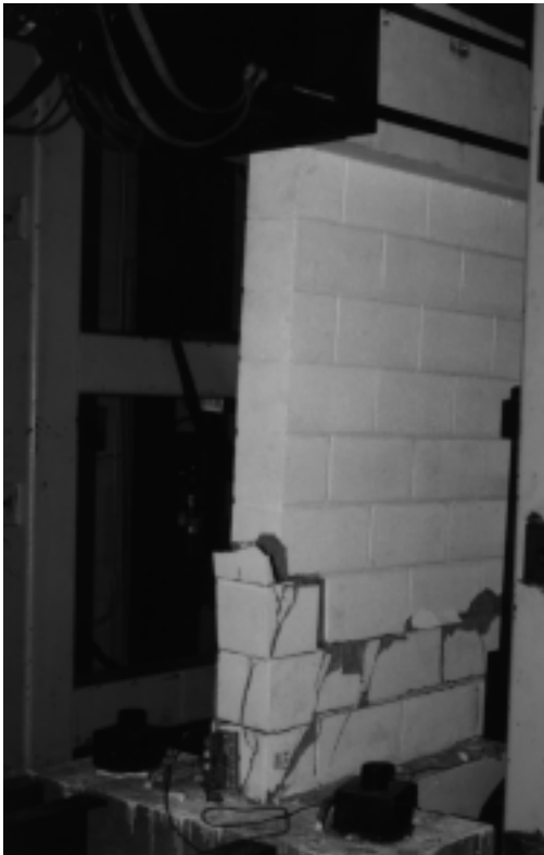
Figure 6. Wall 9 during testing
