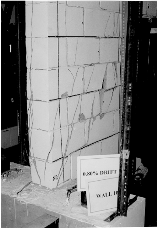
Figure 7. Wall 10: at 0.8% drift, diagonal crushing of masonry
